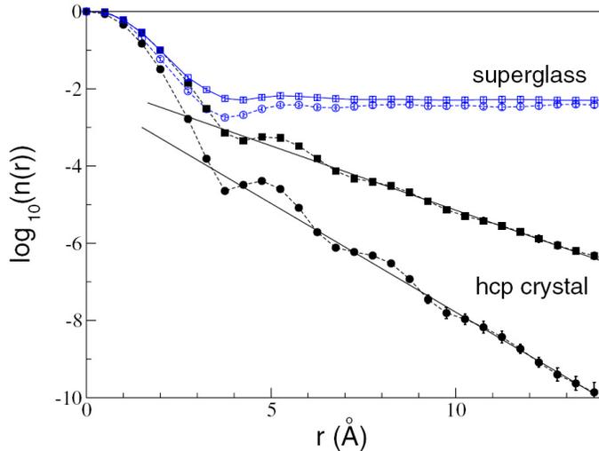
Figure 4: From [14]. The single-particle reduced density matrix  $n(r)$  for the crystalline and “superglass” phases of helium 4, computed from path integral quantum Monte Carlo simulations. The perfect hcp crystal has an exponentially decaying density matrix, meaning there is no phase coherence at long distances. The superglass phase, however, displays off-diagonal long-range order.
