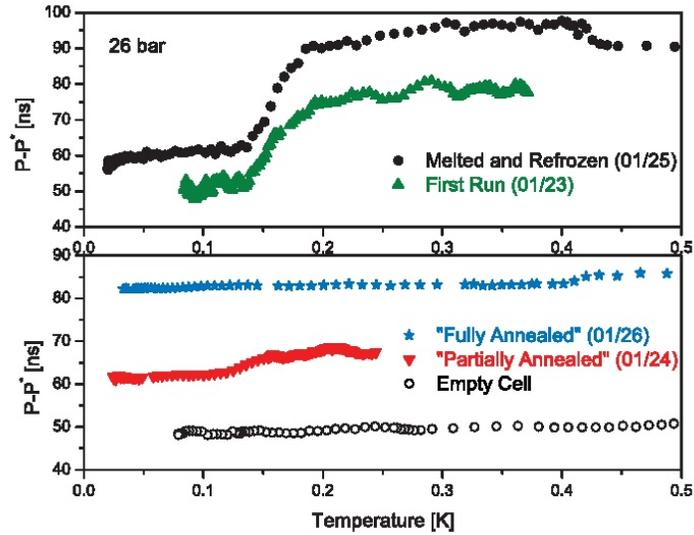
Figure 2: Rittner and Reppy's observation of NCRI [12], showing the effects of annealing. The partially and fully annealed samples have much smaller drops in the resonant period, indicating a strong dependence of NCRI on sample history and defects.
