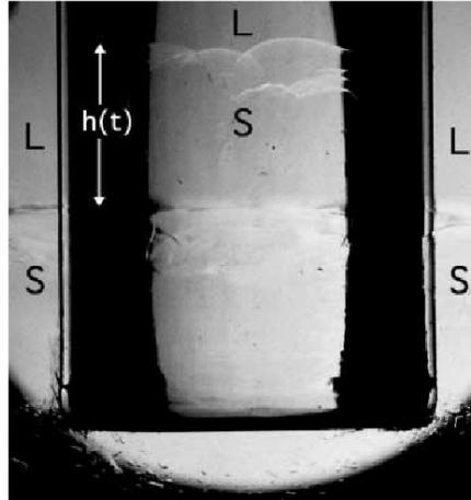
Figure 3: Sasaki *et al.*'s photograph of solid helium in a 1 cm test tube, from Ref. [13]. S denotes solid helium, L denotes liquid helium. The solid-liquid interface is higher inside the tube by  $h(t)$ ; if (and only if) grain boundaries are present, the interface is observed to fall to the outside level.
